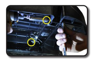
Using quick release pins from hardware pack secure footrest to bagwell bracket as shown.
