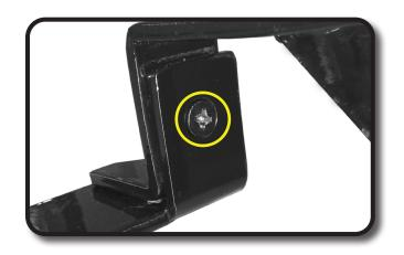
Attach bagwell bracket to cart and support bracket using hardware from Pack 5. For middle hole in support bracket use 8mm hardware, the 2" washer goes underneath the cart.
