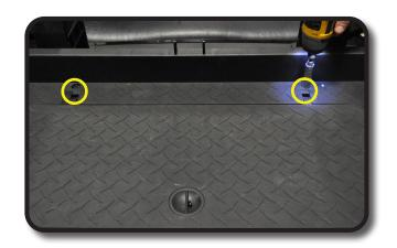
Attach main polyboard frame to bagwell bracket using hardware in Pack 2.
