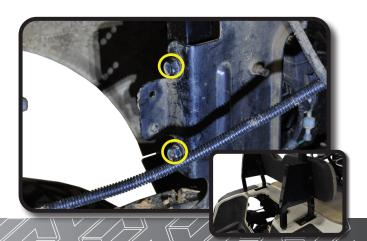
Attach factory struts to seat bracket as shown using hardware retained from Step 1.
